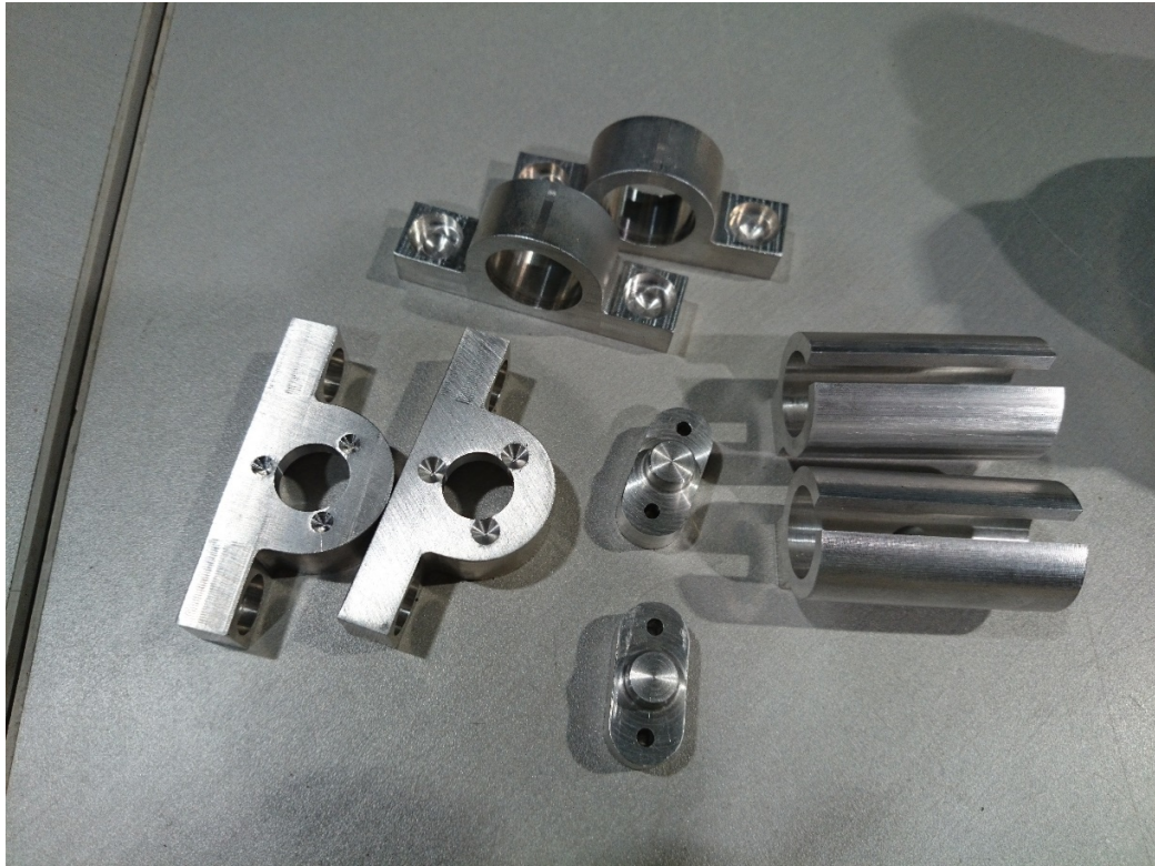
Fig. 4.2. The designs were manufactured in the GUC industrial park in a laser cutter machine, milling and drilling CNC machines
